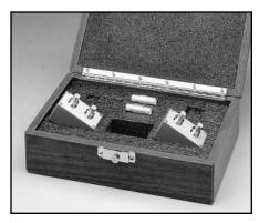
**Model 5907:** Calibration sources to calibrate cable and matrix. Includes 1.8nF and 470pF capacitance sources, 2 BNC female-to-female barrels (CS-565), and 5900-312 storage case.
