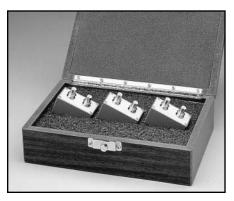
**Model 5955:** Calibration sources for Model 595. Includes 18nF, 1.8nF, 180pF capacitance sources and storage case.
